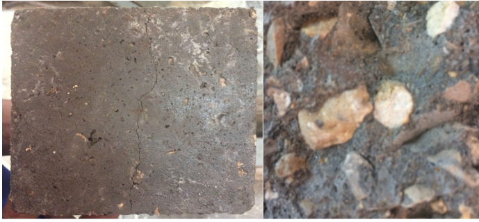
Figure 5. Failure Mechanism of Treated CRC Cube
