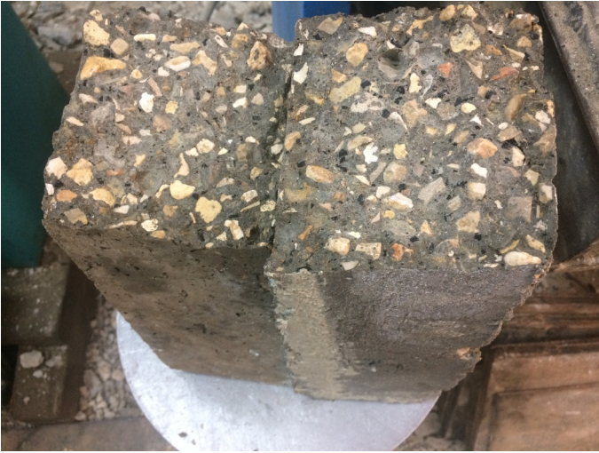
Figure 9. Crack Pattern for Treated Prism
