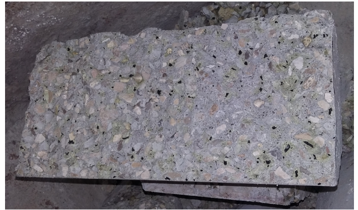
Figure 7. Crack Pattern for Treated Cylinder
